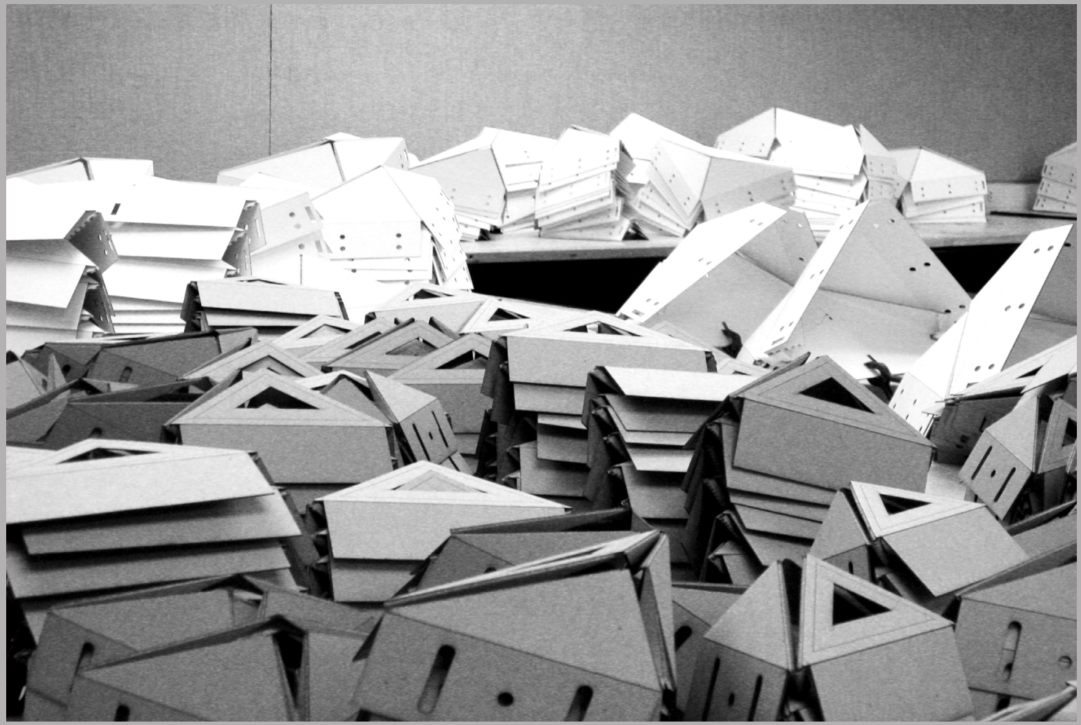
Fig.85. Folded units - units that have been folded prior to receiving the structural frame
