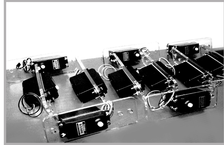
Fig.68. Servo motors - Futaba S3306 servos mounted to plexi
